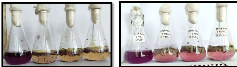
Fig 4 : Decolorization of Methyl violet dye by Aspergillus niger and Aspergillus flavus
